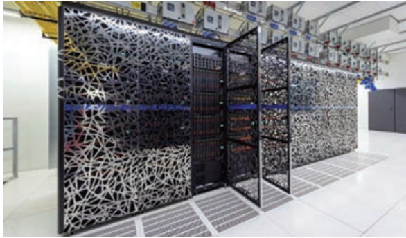
▲ KNMI Supercomputer has a capacity of 50 trillion calculations/sec (50 teraflops). HARMONIE requires around 3 quadrillion calculations.
